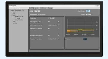
NAPCON Optimizer faceplates are convenient engineer user-interfaces to adjust tuning parameters online.
