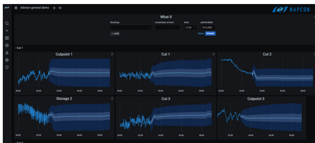
Figure 2. A digital operator assistant predicts the dynamic behaviour of process variables; creates what-if scenarios to allow operators to test various operative scenarios; and suggests what changes should be made in order to meet operation objectives.
