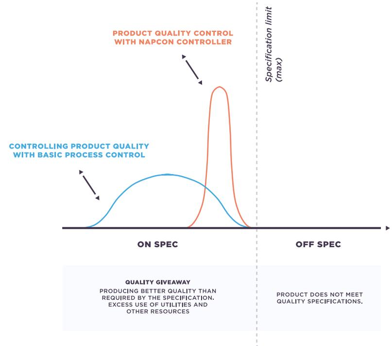
The optimal process operation is to run as close as possible to the process limits. NAPCON Controller decreases variance in main quality variables and keeps the process safely and economically near, but on the right side of the constraints.
