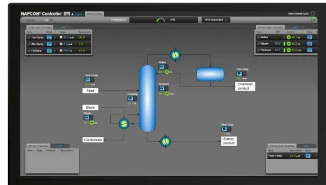
NAPCON Controller operator user interface is based on the latest web technology. It can be seamlessly integrated to all modern DCS or SCADA operating environments and facilitates fluent workflow for panel operators.
